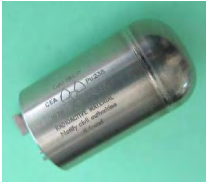
Figure 1 – The nuclear battery developed by Alcatel for Medtronic used a tiny slug of metallic Plutonium 238. The heat produced by the decay of the Pu-238 was converted to electricity by a thermopile.
