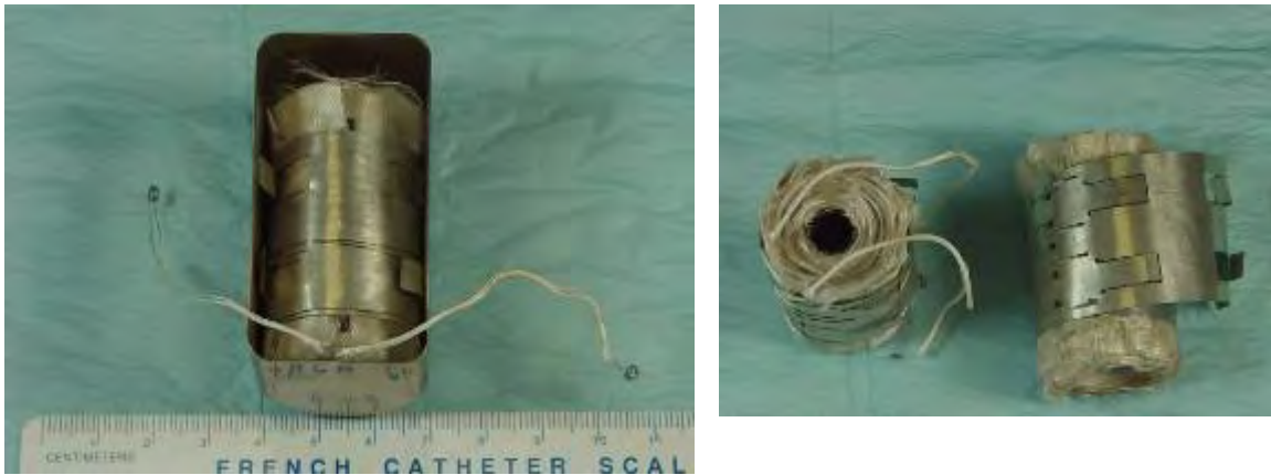
Figure 4 – Thermopiles used in the ARCO Medical pacemaker. The resistance is about 14\text{k}\Omega ohms. ~80 pairs of cupron-tophel thermocouples (isolated with glass tape) in series generate about ~1-2 volts. Six of these tapes are wound together (series/parallel) to make a thermopile. The core of the thermopile is heated with plutonium 238 in a series of capsules. This thermopile was sealed in a vacuum. Photographs courtesy of Paul Spehr who worked at ARCO before it was acquired by Intermedics.
