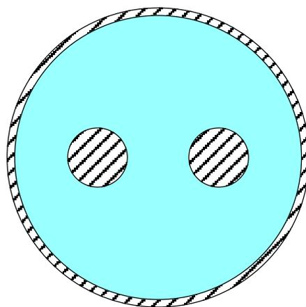
The electrical influence of the surrounding pairs in the cable may be modelled as an equivalent shield. This model will give accurate estimates of  $R$ ,  $L$ ,  $C$  and  $G$  [12]
