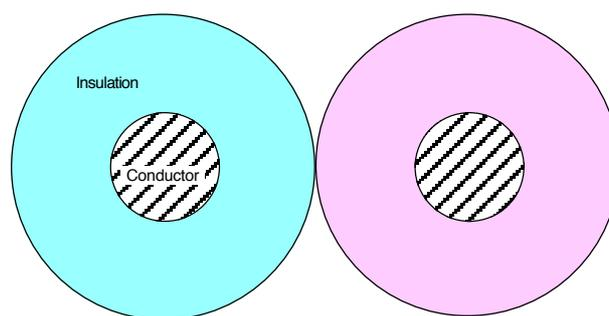
**Most common conductor diameters:** 0.4 mm, 0.6 mm
