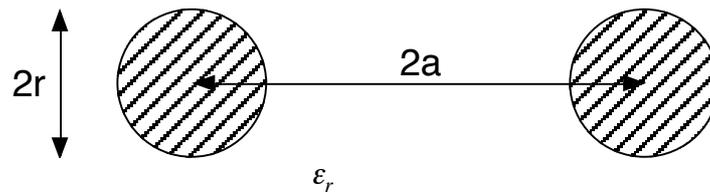
A coarse estimate of the primary parameters  $R$ ,  $L$ ,  $C$ ,  $G$  may be found assuming  $a \gg r$ , uniform insulation, and no surrounding conductors
