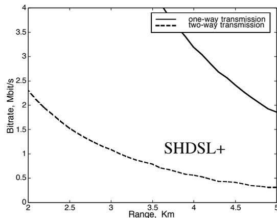
SHDSL+ means a multicarrier system using approximately the same frequency band as SHDSL
