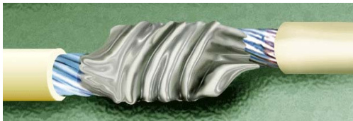
Figure 19-10. Soldered Lash Splice
