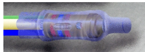
Figure 19-24. Contact Covered With Shrink Sleeving
