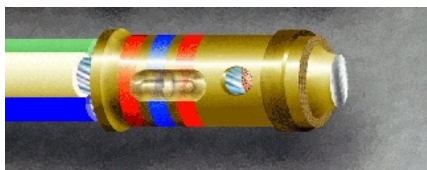
Figure 19-23. Contact Trimmed and Deburred
