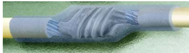
Figure 19-11. Sleeved Lash Splice
