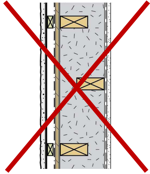
2x4 Double Stud Wall on 2x6 with Staggered Overlapping Studs (It is also nearly impossible to reach R-22 without a gap between the two stud walls)
