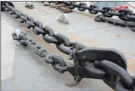
Anchor chain with chain stopper and pelican hook
