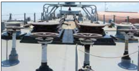
Port outer wheel is the port capstan/wildcat speed control. The port inner wheel is the brake. Same arrangement on starboard
