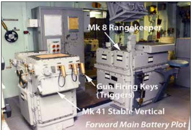
Forward main battery plot room (16-inch guns)
