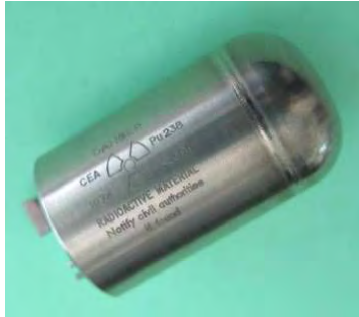
Figure 1 – The nuclear battery developed by Alcatel for Medtronic used a tiny slug of metallic Plutonium 238. The heat produced by the decay of the Pu-238 was converted to electricity by a thermopile.
