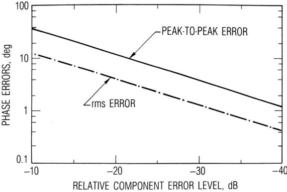
Figure 1-12 Coherent error statistical values [5] (©1989 IEEE)
