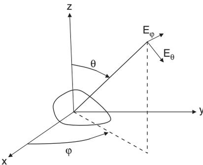
Figure 1-1 Coordinate system for aperture antennas
