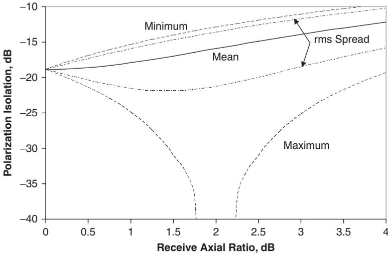
Figure 1-7 Polarization isolation statistics
