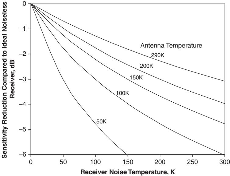
Figure 1-16 Sensitivity reduction from receiver noise temperature
