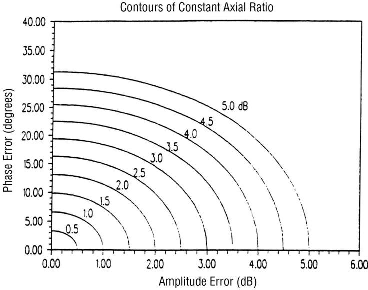
Figure 1-8 Hybrid imbalance impacts on axial ratio [4] (©1990 IEEE)
