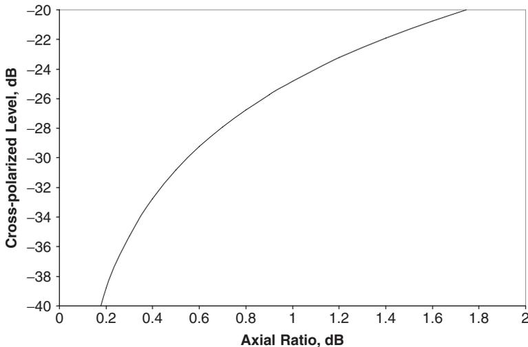
Figure 1-5 Cross-polarized level versus axial ratio
