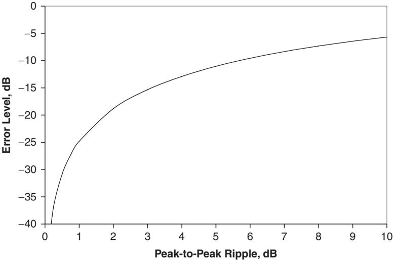
Figure 1-13 Error component level versus peak-to-peak ripple
