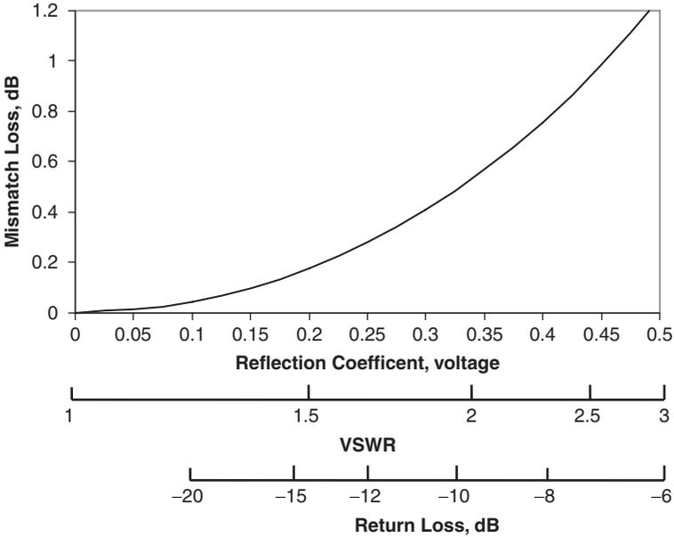
Figure 1-9 Impedance mismatch loss versus common impedance parameters
