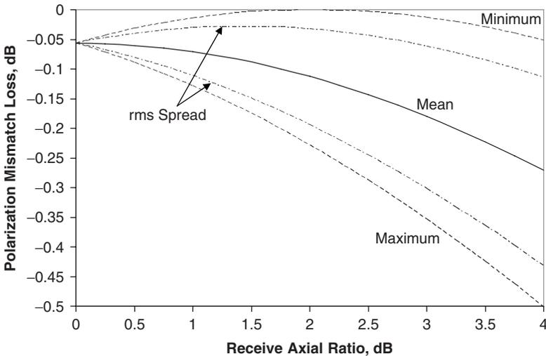
Figure 1-6 Polarization mismatch loss statistics
