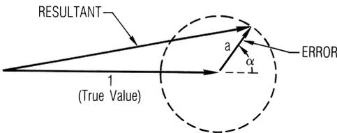
Figure 1-11 Phasor diagram for coherent errors [5] (©1989 IEEE)
