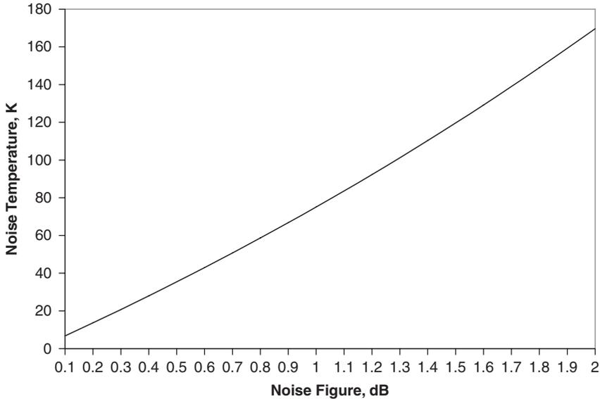
Figure 1-15 Noise temperature versus noise figure
