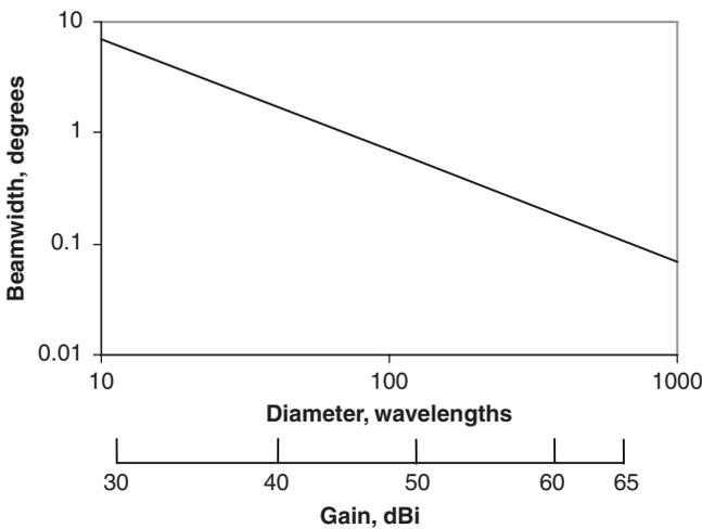
Figure 1-2 Nominal antenna gain and beamwidth values
