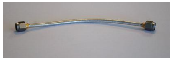
Figure 3: Conformable SMA-SMA cable
