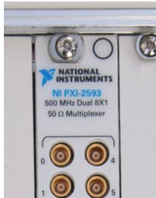
Figure 11. Single-slot PXI module with female MCX connectors
