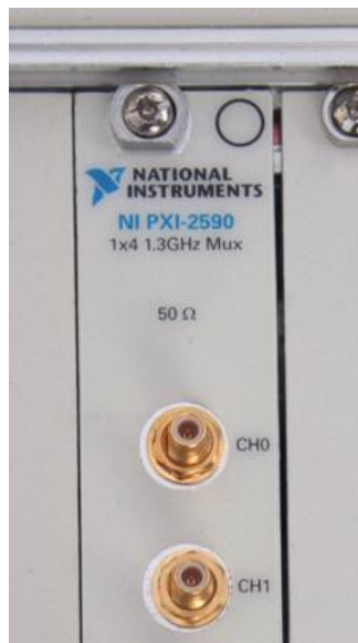
Figure 8. Single-slot PXI module with male SMB connectors
