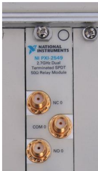
Figure 7. Single-slot PXI module with female SMA connectors
