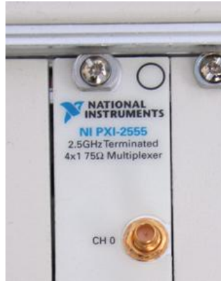
Figure 10. Single-slot PXI module with male mini-75 Ohm SMB connectors
