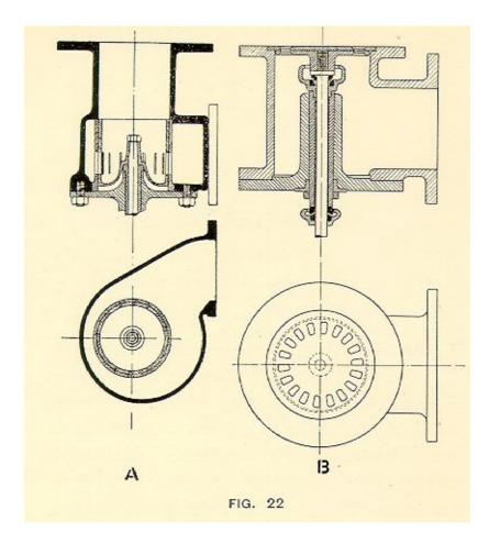
A form analogous to the siren is the "Diaphone." In this a cylinder having circular slits in it, is given a reciprocating motion under the action of compressed air.
