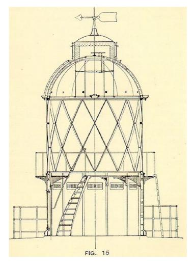
For cleaning the glazing, galleries run round the lantern inside and out, and ladders are provided for reaching the top panes. A copper dish (F), is provided just below the ventilator to catch any water which may possibly be driven through the latter; the heat from the burner below very soon evaporates this.
