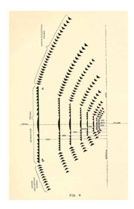
Mirrors.—As explained above, those of the paraboloid form, for reflecting the rays in a parallel beam, are nearly obsolete for Lighthouse purposes, but **Spherical Mirrors** are largely used to reflect rays, which would otherwise be lost, back to the source of light, thus strengthening the effect of the latter, through which they pass, and are refracted or reflected with the other rays in the direction required.
