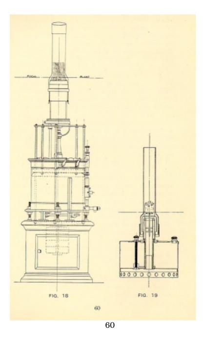
The former type *(a)* gives comparatively high candle powers, and is for use in large lights, but has now been practically superseded by the incandescent oil burner, and is seldom supplied except as a "Standby" to the latter.
