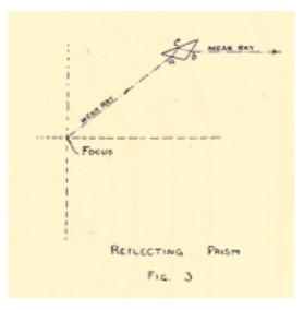
The ordinary Lighthouse Apparatus (see Fig. 4) which consists of refractors over the central portion of its vertical section (from **b** to **c** in Fig. 4), and reflecting prisms over the rest, is, strictly speaking, Catadioptric, as it uses both reflection and refraction, but in modern parlance it is usual to refer to any apparatus consisting of glass elements only as Dioptric."
