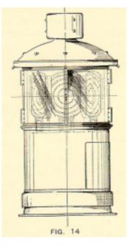
With regard to the illuminant to be used in such Lights, for ordinary positions, the simplest is a wick burner of the capillary type, which can be left unattended all night, and gives a very satisfactory result. For positions which are close to or in a
