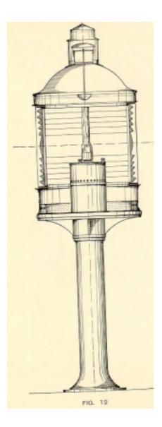
Port-Lights can be arranged for hoisting, so as to exhibit them at night at the top of a mast, and lower them for convenience of cleaning during the day (see Fig. 13).
