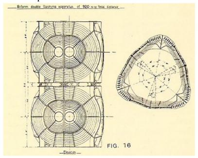
As many as four apparatus have been superimposed, but in this case each is a Lens Light only.
