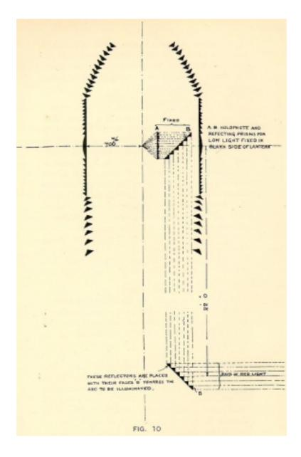
of 1 3/4 miles. It will be noticed that the rays from the portion of the apparatus which shows the red sector are arranged to cross each other; the object of this is to allow of the window opening being narrower than would otherwise be possible, thus avoiding weakening the tower.
