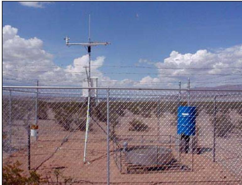
**Figure 5. Class A Evaporation Pan at Elephant Butte Reservoir**
