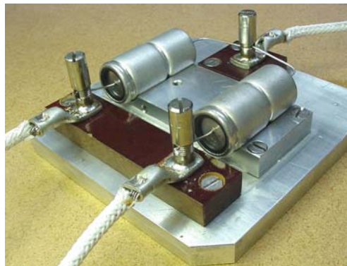
Test set-up, capacitors mounted with low thermal resistance path, to metallic chassis:
