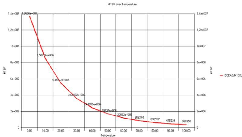
Figure 1. Plot of MTBF vs Temperature for an aluminum electrolytic capacitor – generic application – GM (Ground Mobile) MIL HDBK 217 model
