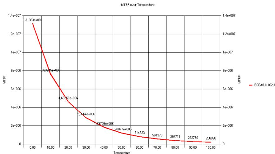
Figure 2. Plot of MTBF vs Temperature for an aluminum electrolytic capacitor – generic application – GM (Ground Mobile) TELCORDIA model.
