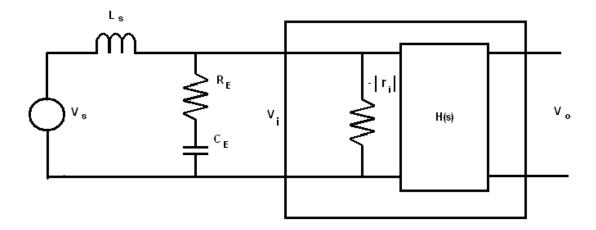
Compared to the previous schematic, the resistance  $R_S$  has been removed to simplify the analysis. This is, in general, an advantage, because a resistive element in series with the input lead causes power dissipation and penalizes the overall efficiency. The resistance  $R_E$  is the equivalent series resistance (ESR) of the capacitor  $C_E$ .
