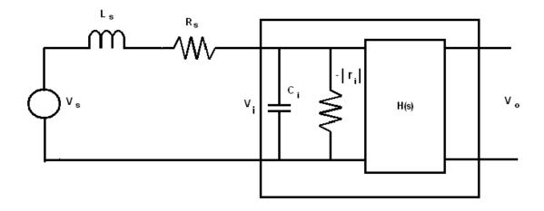
Here, the negative incremental input impedance is indicated as  $-|r_i|$ . Further, an additional internal capacitor  $C_i$  has also been added, as this is the typical case, at the input stage of a DC/DC converter.
