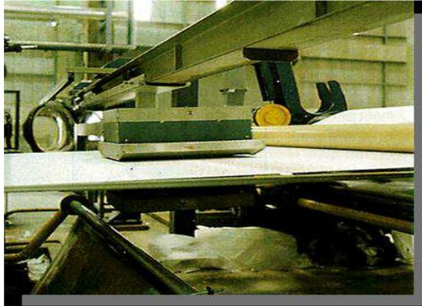
*FIG. VI-3. Thickness gauge used in paper production. Typical sources include:  $^{90}\text{Sr}$  (370 MBq (10 mCi) to 3.7 GBq (100 mCi));  $^{85}\text{Kr}$  (370 MBq (10 mCi) to 18.5 GBq (500 mCi));  $^{147}\text{Pm}$  (3.7 GBq (100 mCi) to 18.5 GBq (500 mCi)).*
